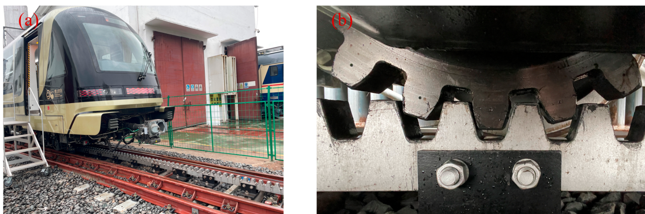
Figure 1. Mountain rack train test line: (a) mountain rack train; (b) gear–rack traction system.
