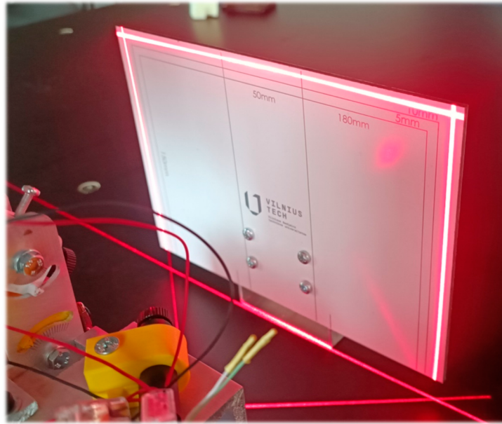
Figure 8. Calibration plate for laser scanner.
