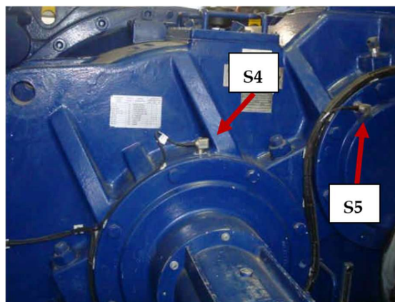
Figure 3. Photograph showing the location of the vertical accelerometer (S4) and axial accelerometer (S5) on the gearbox near the ISS and HSS, viewed from the generator.
