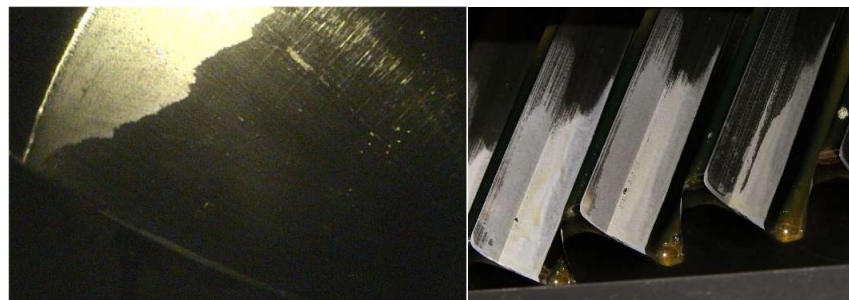
Figure 5. Pitting (left) and wear (right) on the pinion gear mounted on the ISS.
