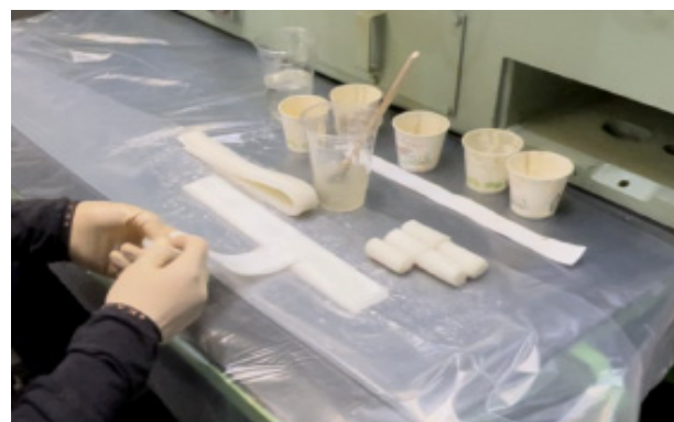
Figure 20. Preparation of polyester (HP21) insulation reinforcement material.
