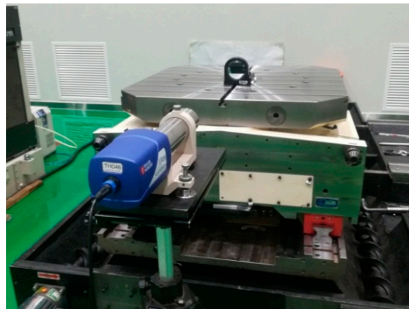
Figure 12. Measurement for X-axis integrated error of the \mu 2000/800\text{H} horizontal machining center.
