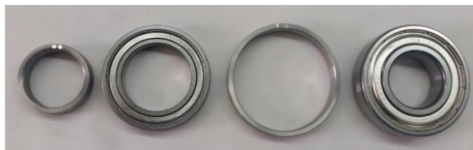
Figure 10. From left to right: inner ring, new ball bearing, outer ring, original ball bearing.
