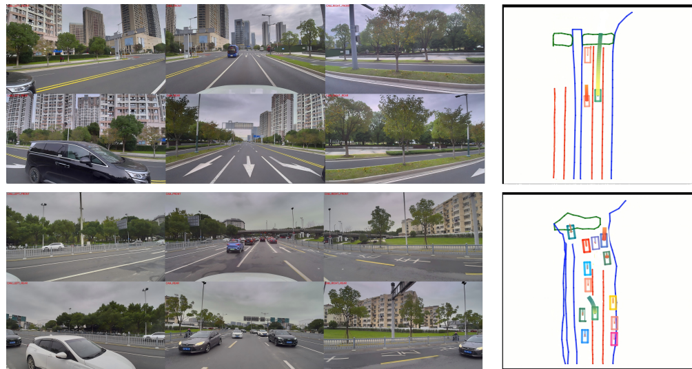
Figure 7. Visualization of OAIAD's results on the real-world dataset. The top row shows planning results for the occlusion scenarios, while the bottom row illustrates the results for lane-change interaction scenarios. The green box and trajectory represent the ego vehicle.
