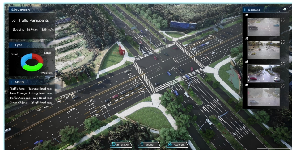
(b) Visualization of the vehicle–road–cloud collaborative system, used to provide ground-truth labels, contains objects, maps, and trajectories.
