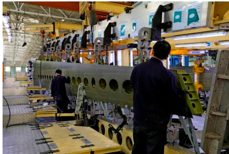
Figure 1. Manual assembly operation inside the wing-box.
