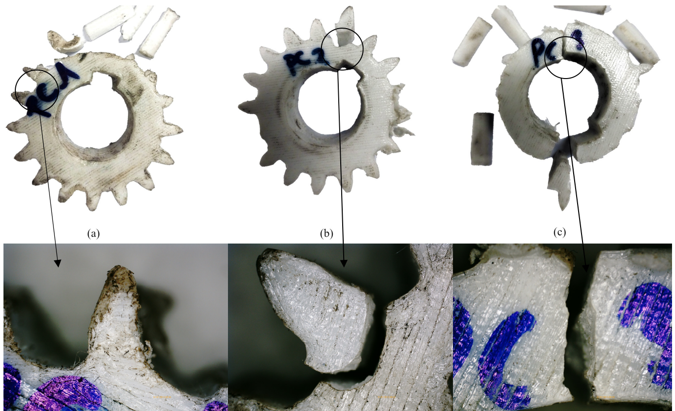
Figure 21. The failure mechanism of PC gear samples: (a) first gear sample; (b) second gear sample; (c) third gear sample.
