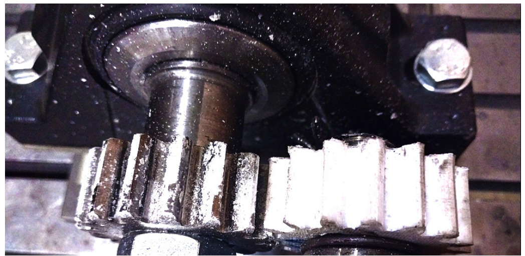
Figure 20. Excessive wear of the PC gear sample after 30 min of testing.
