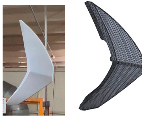
Figure 10. Three-dimensional model and physical body of the motorcycle shell for spraying trajectory tracking.
