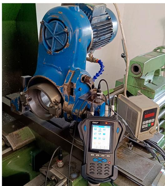
**Figure 5.** Thread whirling attachment and Microlog gx CMXA 75 analyzer.
