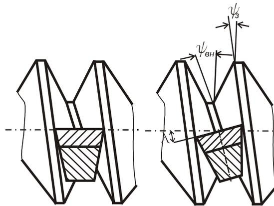
**Figure 7.** Scheme of installing the cutter perpendicular to the inclination of the screw turn: on the **left**—without the inclination of the cutting insert ( $\lambda = 0$ ); on the **right**—with the inclination of the cutting insert ( $\lambda > 0$ ).
