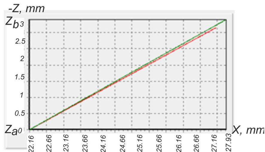
**Figure 18.** Comparison of the models of the side profile  $AB$  of the NC23 thread: standard (red) and made using the cutting tool with the geometric parameters of  $\gamma = 12^\circ$ ,  $\lambda_z = 2.61^\circ$  (green).
