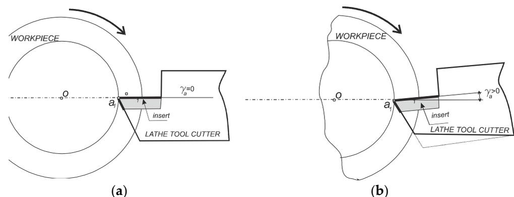
**Figure 6.** The scheme of ensuring the specified value of the back-rake angle  $\gamma$ : (a) conventional tool with back-rake angle  $\gamma = 0$ ; (b) modernized tool shank with a changed tool base with back-rake angle  $\gamma < 0$ .
