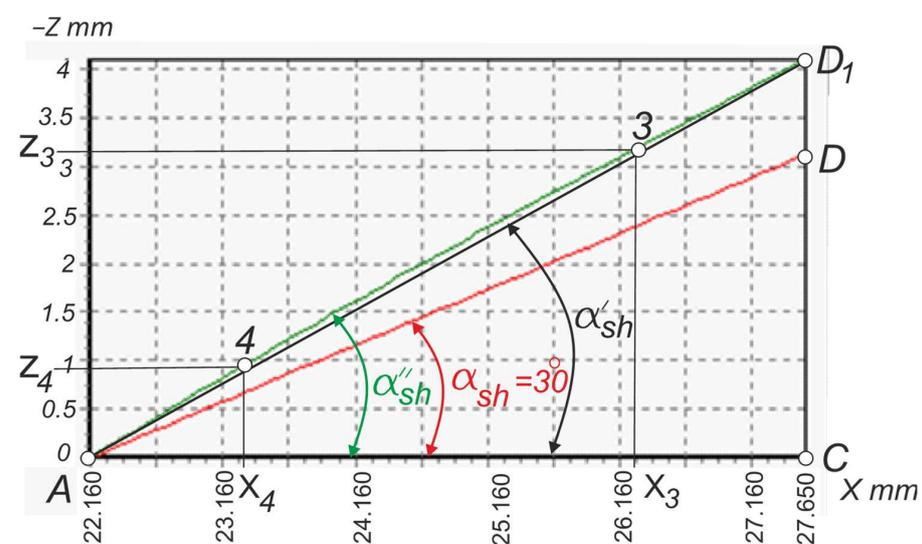
**Figure 17.** Comparison of models of the side profile of the NC23 thread: red straight  $AD$ —standard; green curve  $AD_1$ —predicted profile obtained using the tool with geometric parameters of the cutter  $\gamma = 50^\circ$ ,  $\lambda_z = 2.61^\circ$ ; black straight  $AD_1$ —linear interpolation of the green curve by two points.
