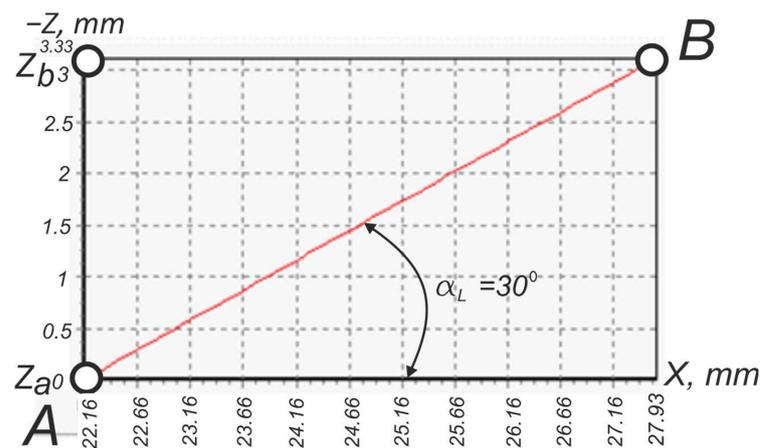
**Figure 15.** Visual software model of the flank profile  $AB$  of the drill-string tool-joint thread NC23.
