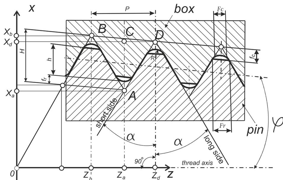
**Figure 1.** Scheme of a drill-string threaded connection according to the API7 standard with reference to the  $ZOX$  rectangular coordinate system:  $H$ —thread height (not truncated);  $h$ —thread height (truncated);  $fr$ —root truncation;  $fc$ —crest truncation;  $R$ —root radius;  $P$ —pitch.
