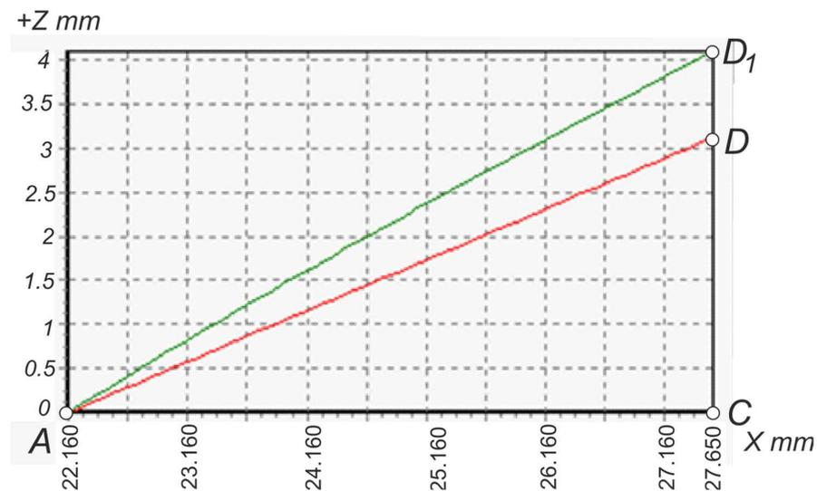
**Figure 16.** Comparison of models of the lateral theoretical profile of the NC23 thread: standard (red) and made by the tool with the geometric parameters of the cutter  $\gamma = 50^\circ$ ,  $\lambda_z = 2.61^\circ$  (green).
