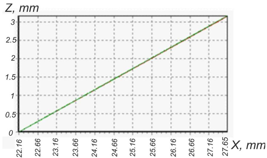
**Figure 19.** Comparison of the models of the side profile AD of the NC23 thread: standard (red) and made using the cutting tool with the geometric parameters of  $\gamma = 12^\circ$ ,  $\lambda_z = 2.61^\circ$  (green).
