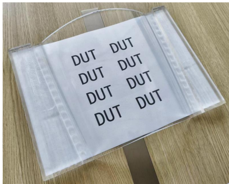
Figure 16. Optical performance of polished complex curved PMMA part.
