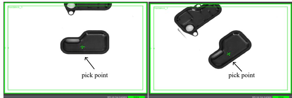
**Figure 5.** Definition and identification of the part's pick-up point based on the changing position and orientation of the buffer.
