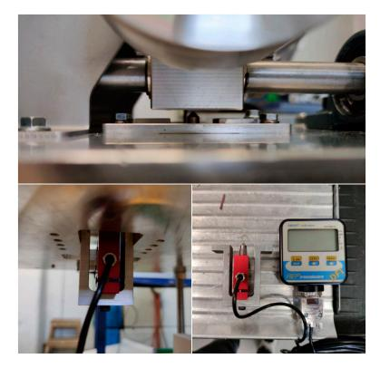
Figure 6. Load cell for torque measurement.
