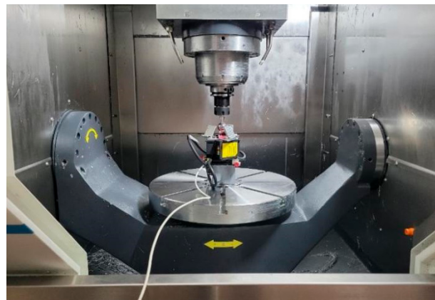
Figure 11. Test setup for the three-dimensional displacement calculation accuracy.
