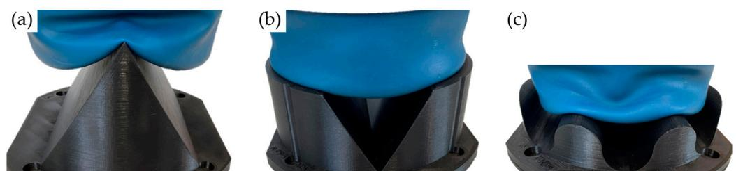
**Figure 8.** Example images of the gripper placed on different extreme ungraspable geometries: (a) convex shape (60° edge), (b) concave shape (60° edge), (c) structured convex/concave surface.
