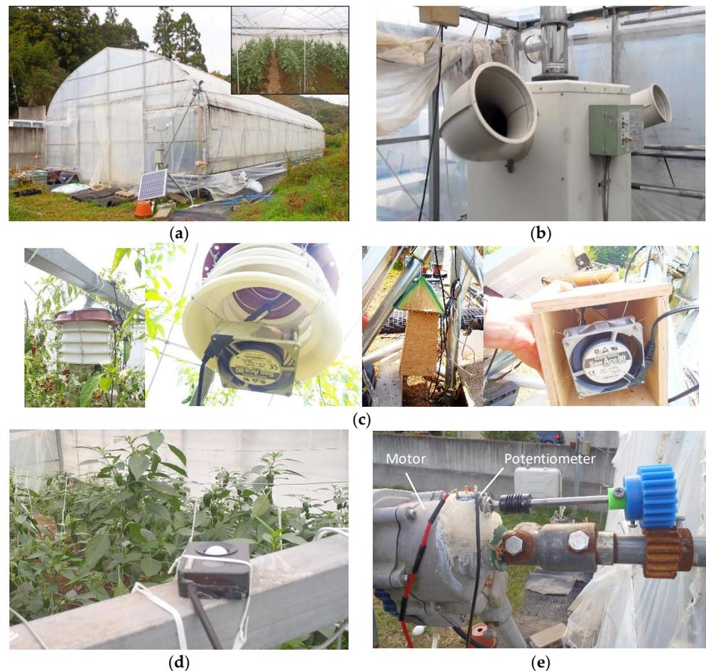
**Figure 1.** Experimental environment: (a) green pepper greenhouse facility; (b) boiler; (c) temperature and humidity sensor in the ventilator (left: inside the house; right: outside the house); (d) illuminance sensor; (e) vinyl roll-up skylight opening/closing motor and window-opening sensor.
