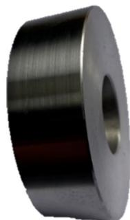
**Figure 13.** The gear blank before gear hobbing.
