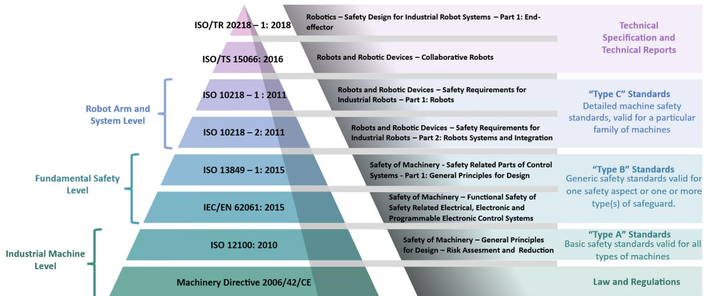
Figure A1. International Standards for the Safety of Human–Robot Collaboration.
