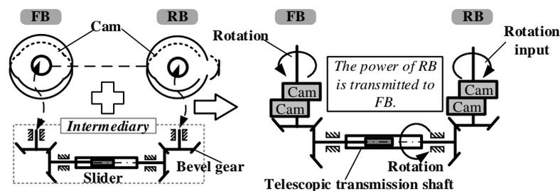
Figure 13. Intermediary—telescopic transmission shaft.
