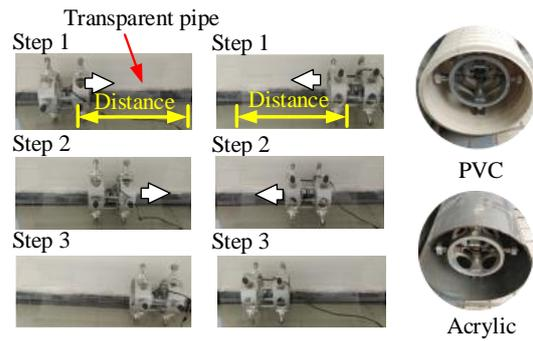
Figure 17. In-pipe robot prototype test of forward and reverse motion.
