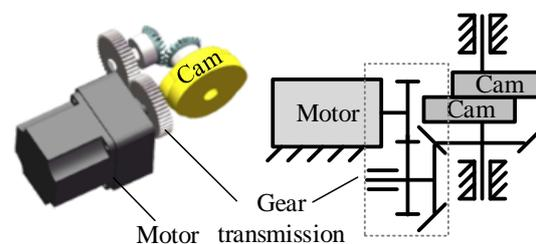
**Figure 10.** Motor-driven cam.
