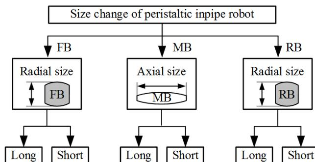
Figure 8. Size change in the peristaltic in-pipe robot.
