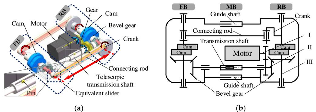
Figure 5. Propulsion mechanism of the novel in-pipe robot. (a) 3D; (b) 2D.
