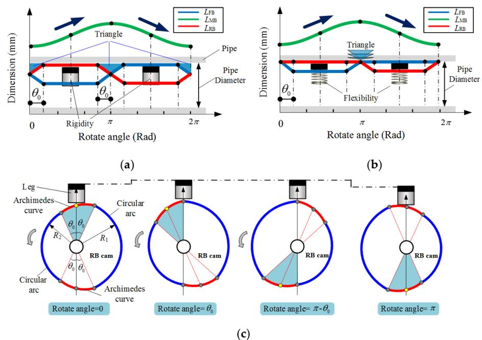
**Figure 16.** Dimension changes when RB cam rotates: (a) rigid leg without spring; (b) elastic leg with spring inside; (c) RB cam rotation status.
