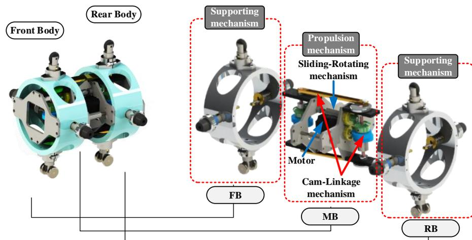
Figure 3. 3D rendering of the novel peristaltic in-pipe robot.
