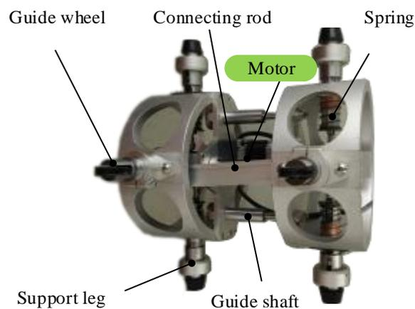
Figure 4. Novel in-pipe robot prototype.
