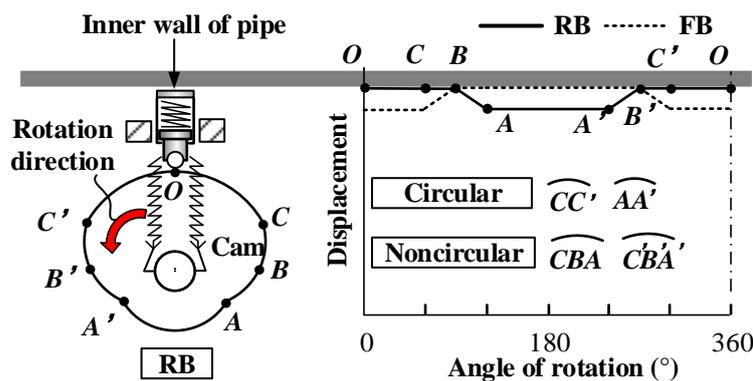
Figure 11. Periodic action of the cam.
