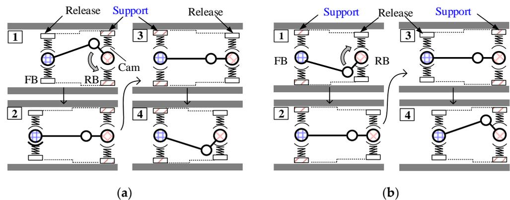
**Figure 6.** Principle of forward and reverse walking: (a) forward walking; (b) reverse walking.
