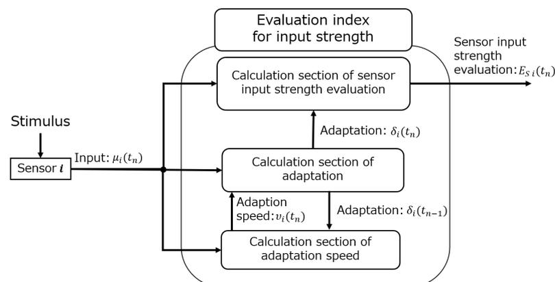
Figure 1. Flowchart depicting an evaluation of the strength of inputs using the proposed method.
