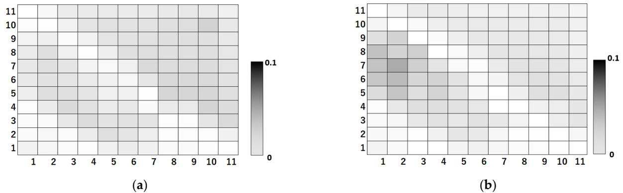
**Figure 7.** (a) Percentage of robot visits to the environment from the first trial to the 500th trial in the previous method; (b) percentage of robot visits to the environment from the 1501st trial to the 2000th trial in the previous method.
