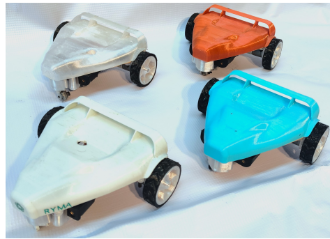
Figure 4. Custom-made differential-drive robots used for experimentation.
