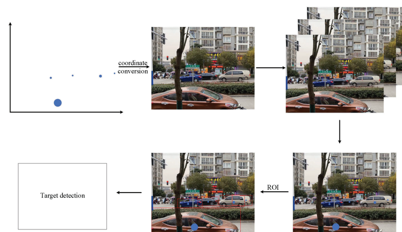
Figure 11. Data-level-based image and radar data fusion [2].
