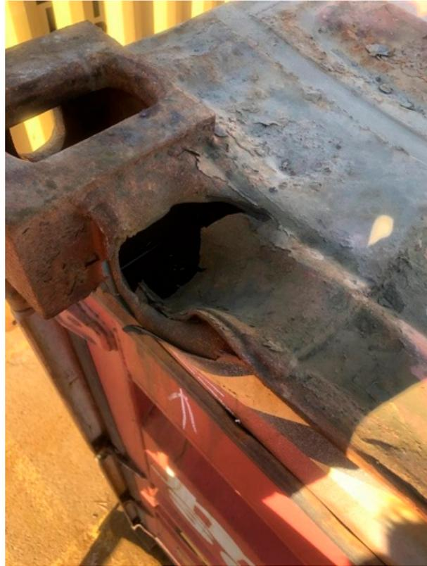
**Figure 1.** The result of the continuous forceful impacts of the spreader hooking mechanisms due to the lack of proper spreader control changes the trajectory of movement of the hooking rods.
