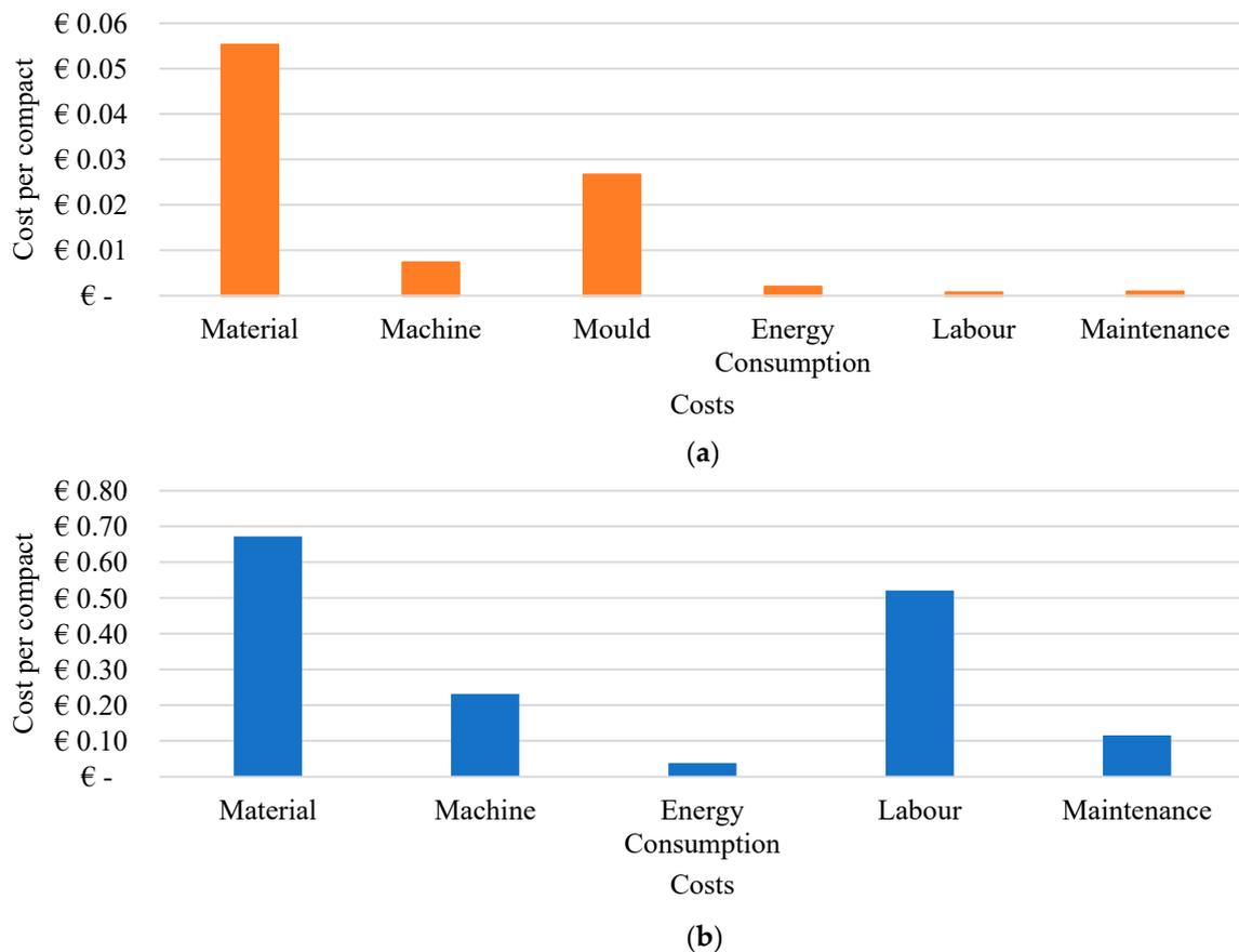
**Figure 4.** (a) IM and (b) FFF cost per compact breakdown.
