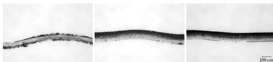
Figure 7. Microscopic displays of fine printed lines obtained by Plate B after varied UV post-treatments (magnification of 50\times ): (left) —2 min of UVA and 10 min of UVC, (middle) —10 min of UVA and 10 min of UVC, (right) —10 min of UVA and 20 min of UVC.
