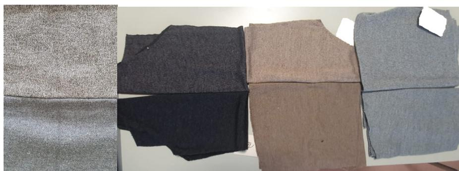
**Figure 1.** Samples with acrylic yarns of different origins, where different shades can be observed (especially dark colors corresponding to Dralon samples) after dyeing.
