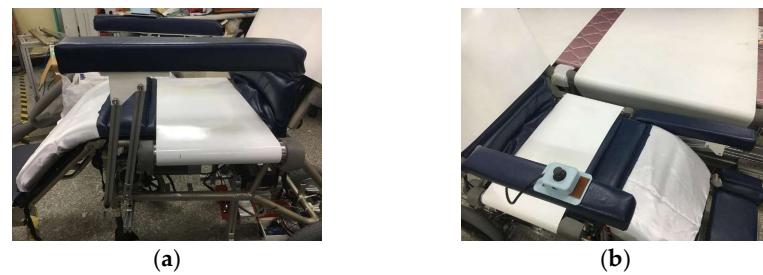
Figure 7. (a) Hand rest in the normal position. (b) Hand rest in the lowest position.
