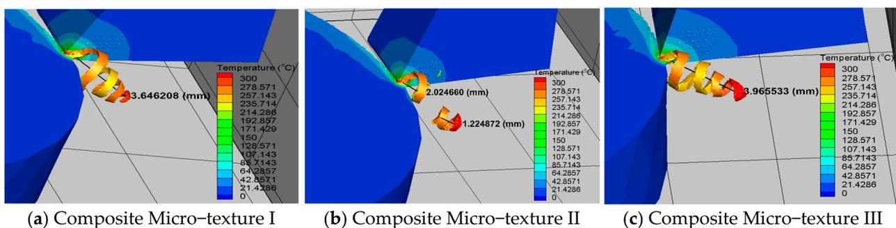
Figure 8. Chip morphology of three composite micro-textured tools.
