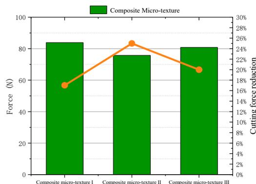
**Figure 11.** Cutting force of composite micro-texture tool.
