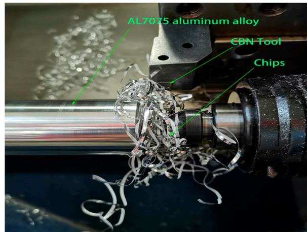
Figure 3. Chip winding.
