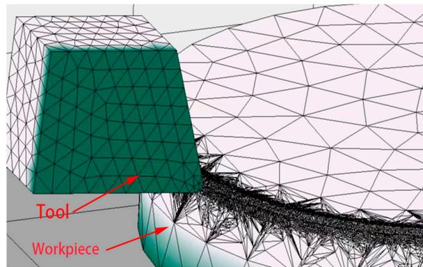
**Figure 7.** Finite element simulation model.
