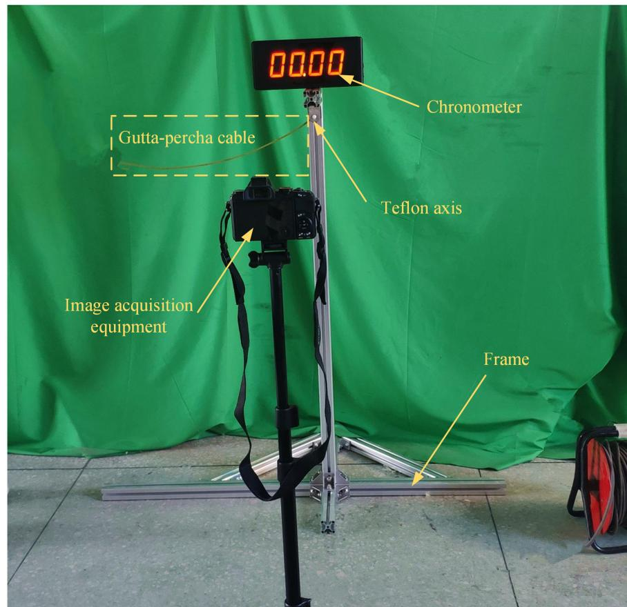
**Figure 9.** The structure of experimental facilities.
