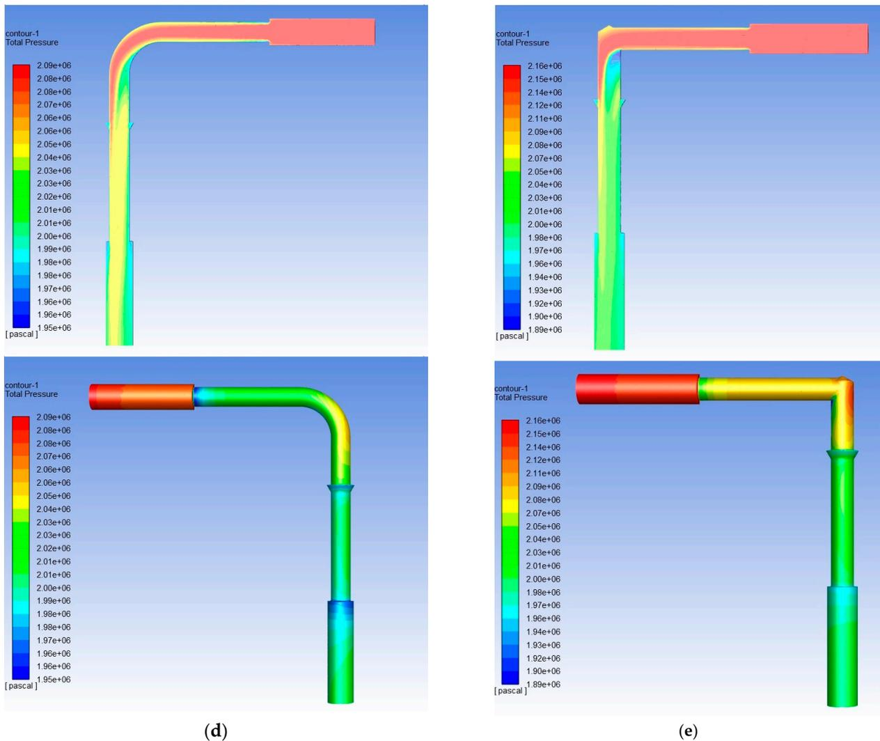
**Figure 7.** View of the total fluid flow pressure across angular fitting connections (top—symmetry side; bottom—wall side): (a) equivalent length method; (b) DKR 45° connection; (c) DKR 45°K connection; (d) DKR 90° connection; (e) DKR 90°K connection.
