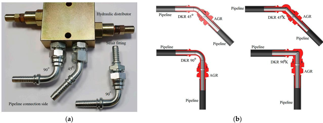
**Figure 2.** Fittings used in the research: (a) Connection of angular fittings in a hydraulic system; (b) Cross-section of angular fitting connections in 3D pipelines models.
