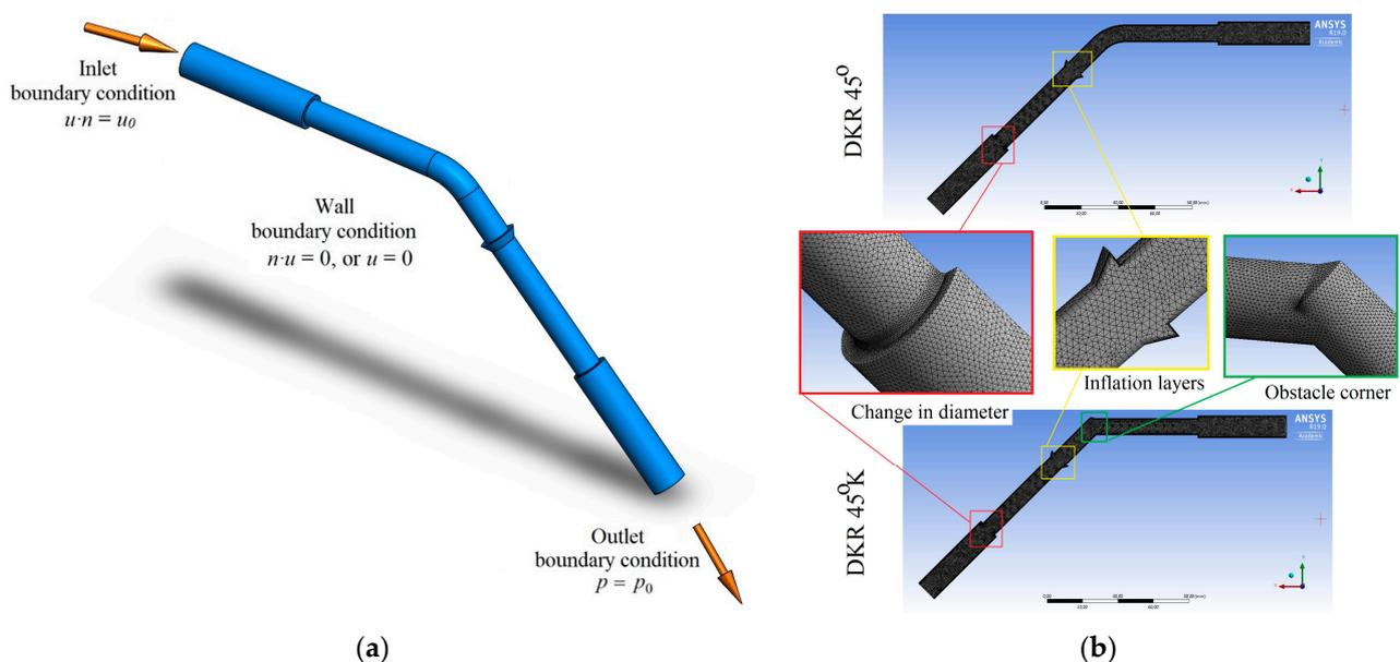
**Figure 4.** Views of the numerical simulation model for angular fitting connections (1/2): (a) boundary conditions of the fluid flow for ANSYS fluent simulation; (b) example mesh of the numerical model.
