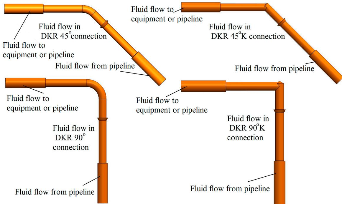
**Figure 3.** Model of fluid flow in the connections of angular fittings in pipelines.
