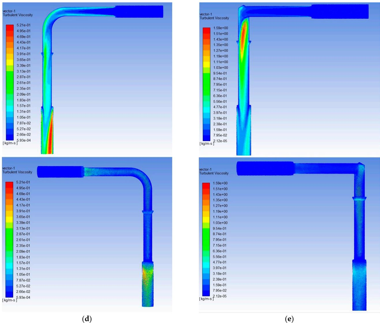
**Figure 8.** View of the fluid flow turbulence processes across angular fitting connections (top—symmetry side; bottom—wall side): (a) equivalent length method; (b) DKR 45° connection; (c) DKR 45°K connection; (d) DKR 90° connection; (e) DKR 90°K connection.
