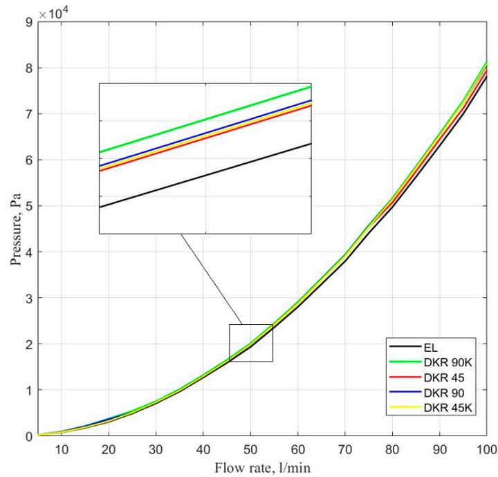
Figure 9. Fluid pressure losses at the angular fitting connections.
