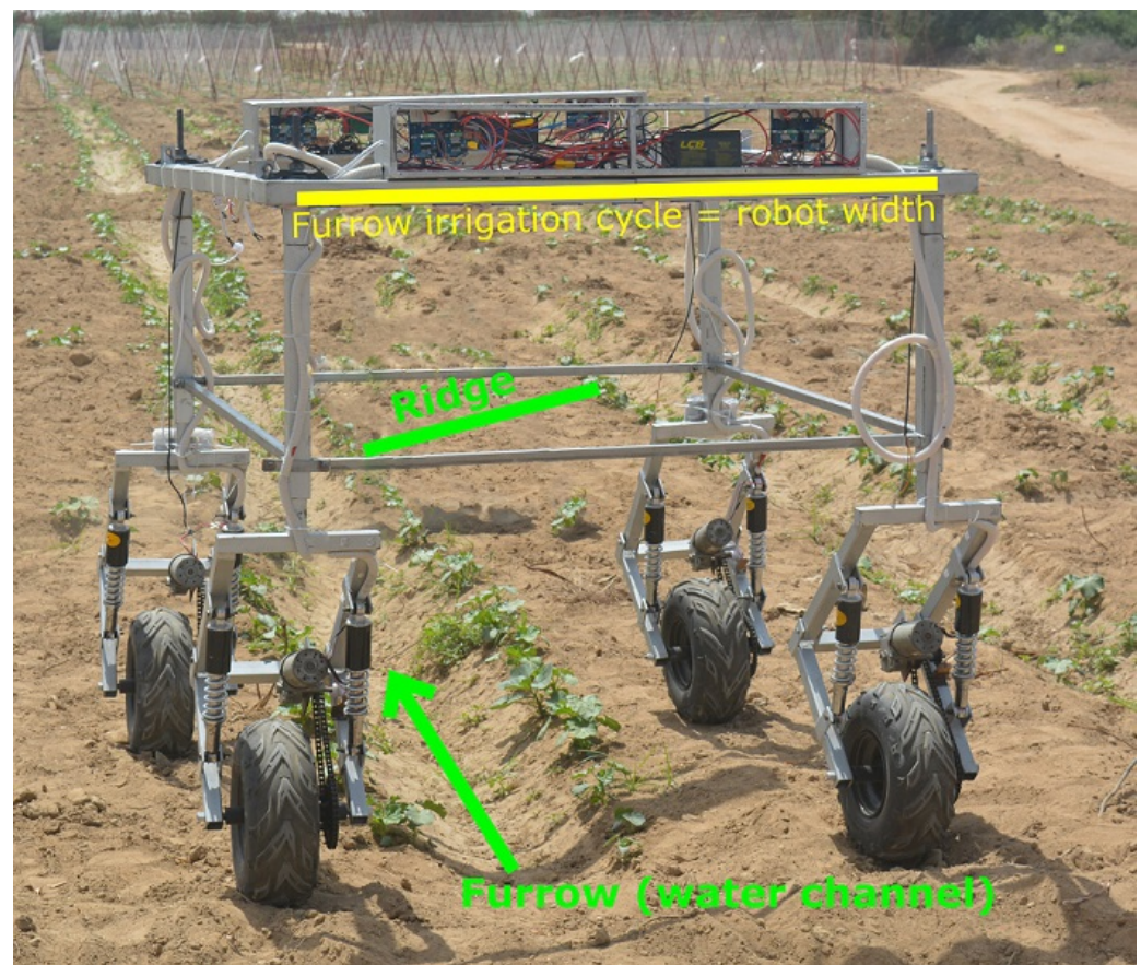
Figure 8. Weed robot dimensions in relation with field cycle
