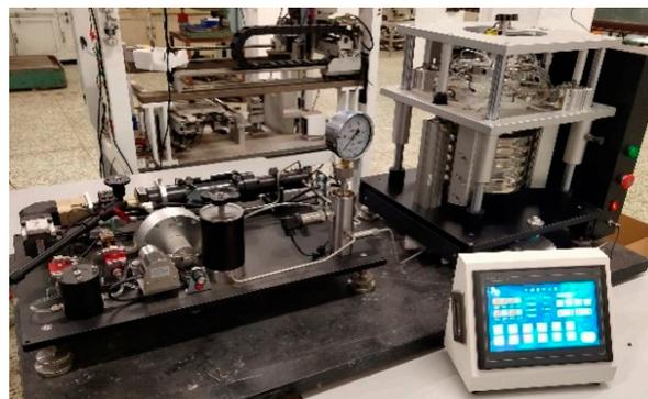
Figure 13. 500 Mpa automatic piston manometer.
