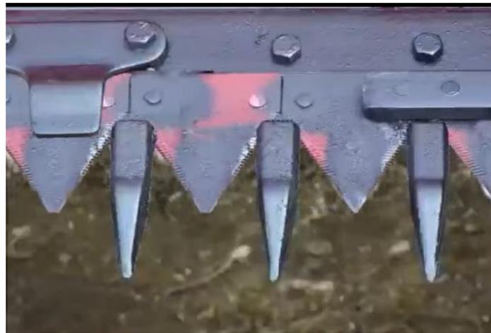
Figure 5. Full-feed combine harvester cutter bar [11].
