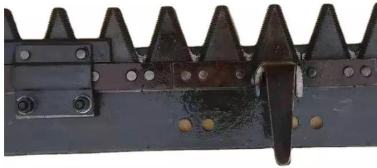
Figure 4. Half-feed combine harvester cutter bar [11].
