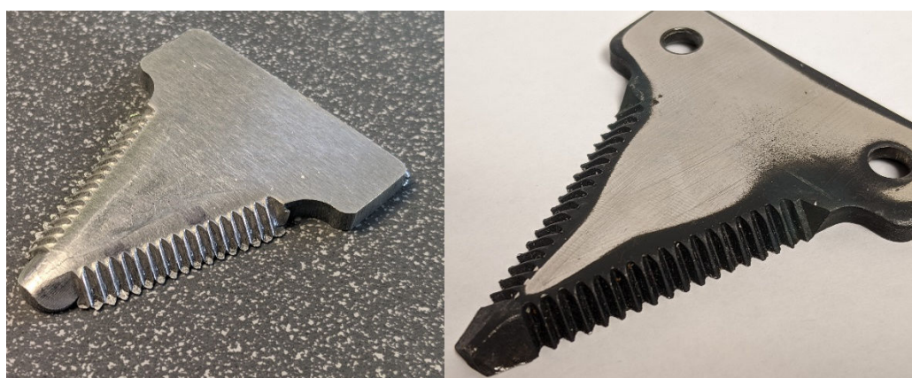
Figure 12. Comparison of the test blade (left) and the original half-feed combine harvester small bottom blade (right).
