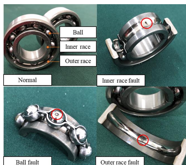
Figure 15. The rolling bearings under four different conditions. The circle is the point of failure.
