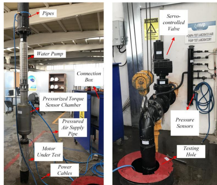
Figure 10. Motor under test, torque sensor, pump assembly, servo-controlled valve, pressure sensor, flowmeter, and testing hole.
