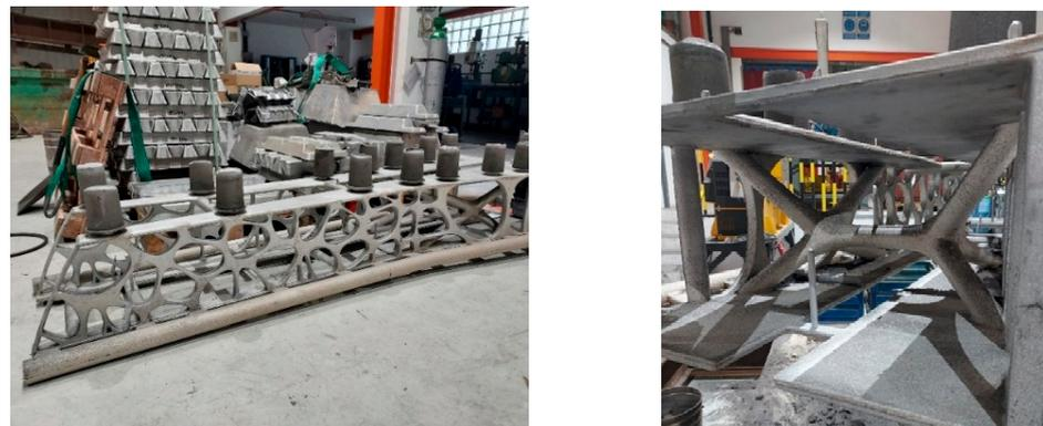
**Figure 17.** Part manufactured after the demolding. Filling and feeding systems are also shown in this image at Tecnia's facilities (left). Inner Skeleton features (right).
