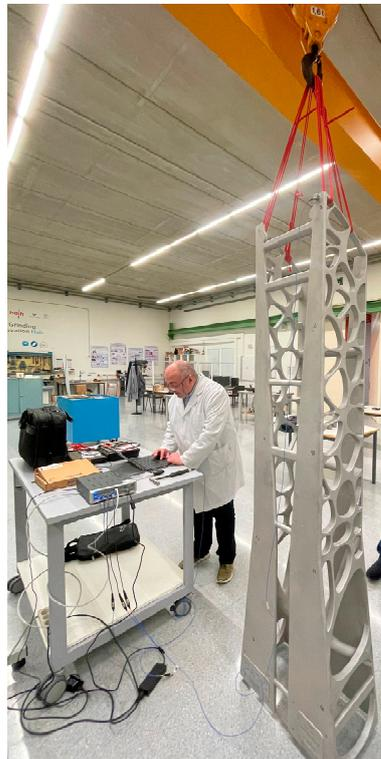
**Figure 18.** Modal test configuration for free vibration conditions with the data-acquisition device, the accelerometer in the top right area of the part, and the hammer at UPV/EHU's facilities.
