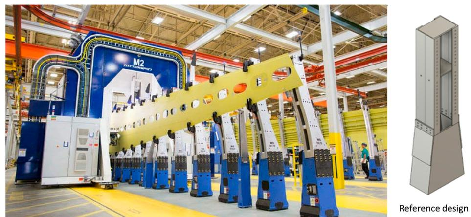
**Figure 2.** The wing skin panels for Boeing’s first 737 MAX airplane are loaded on fixtures into an automated assembly machine in the company’s plant in Renton, Wash., on 2 June 2015 (source: [33]) [left]. The simplified reference design of the assembly column based on the fixtures used in assembly lines [right].
