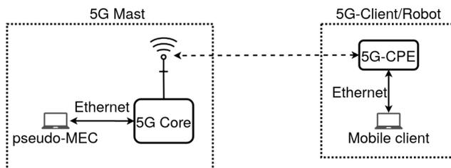
Figure 5. Connection diagram for our 5G-SA network.
