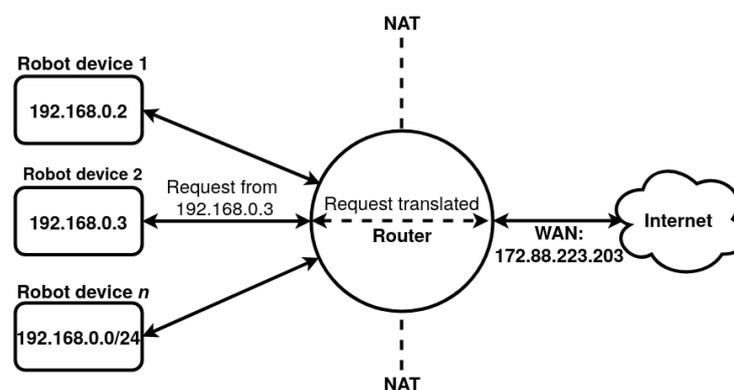
Figure 8. A simplified diagram showing how messages are handled by a router using NAT.
