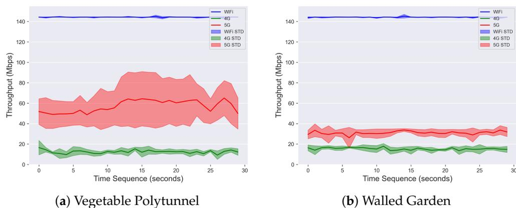
**Figure 10.** Network throughput results, averaged over 5 experimental runs gathered from a single “best” location (please refer to Table 4). The mean is the solid line in the centre of the shaded regions, which shows  $\pm 1$  standard deviation.
