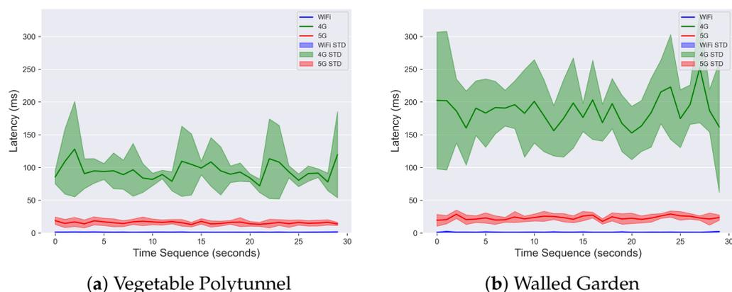
**Figure 9.** Best network latency results, averaged over 5 experimental runs gathered from a single “best” location (please refer to Table 4). The mean is the solid line in the centre of the shaded regions, which shows  $\pm 1$  standard deviation.
