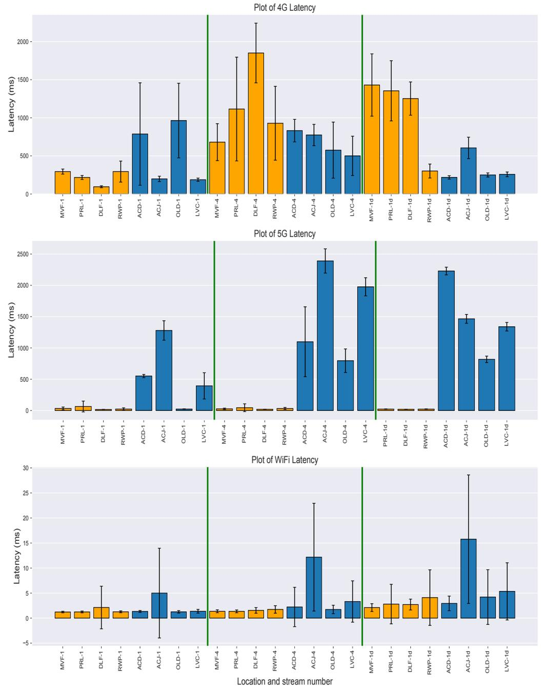
**Figure A1.** Latency results across all performance metrics and parameters. The vertical lines separate the data stream type, and the orange-coloured bars represent the Vegetable Polytunnel and the blue-coloured bars represent the Walled Garden.
