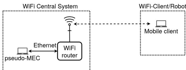
Figure 6. Connection diagram for the WiFi6 network.
