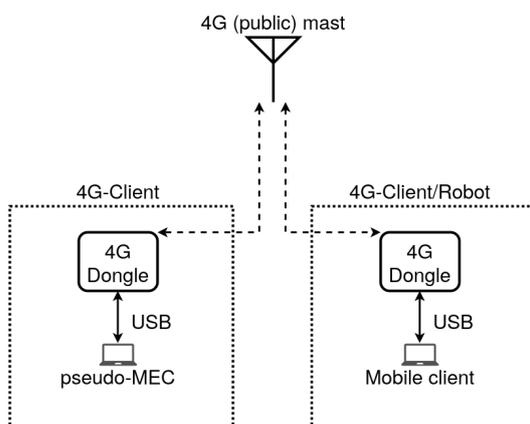
**Figure 7.** Connection diagram for the 4G network.
