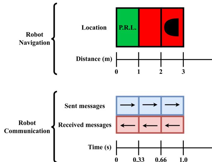
**Figure 12.** Image shows the magnified operation of the simulated robot if it had instantaneous (ideal) communication over a 1 s period.
