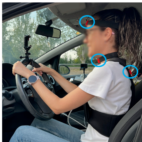
Figure 7. Example of the experimental configuration of wearable units for a test.
