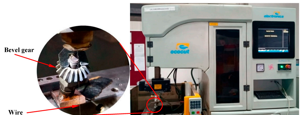
Figure 4. Crack faults created by the CNC wire (EDM) machine.
