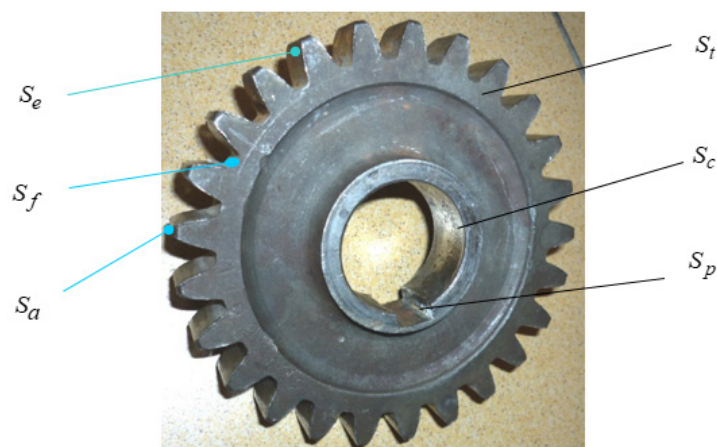
Figure 11. The boundary surfaces of a spur gear.
