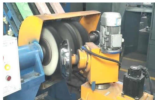
Figure 13. Machining process (CNC polishing machine working process).
