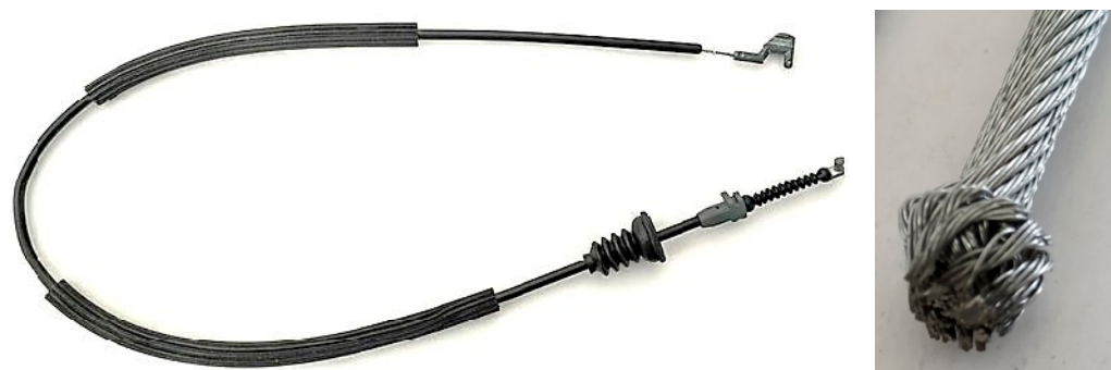
Figure 1. Example of a Bowden cable (left) and a mushroom at the end of the wire rope (right).
