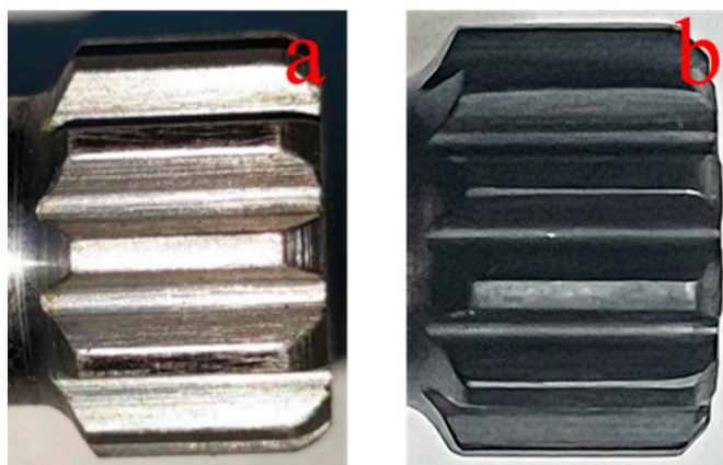
Figure 18. Tooth surface of external spline without wear. (a) External spline without carburizing treatment; (b) external spline with carburizing treatment.
