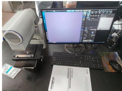
Figure 23. Olympus DSX510 digital microscope.
