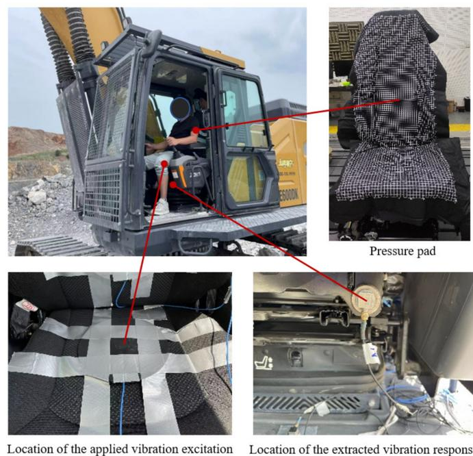
**Figure 6.** Body pressure distribution test and vibration response test.
