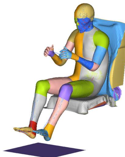
**Figure 5.** Human-seat coupling finite element model.
