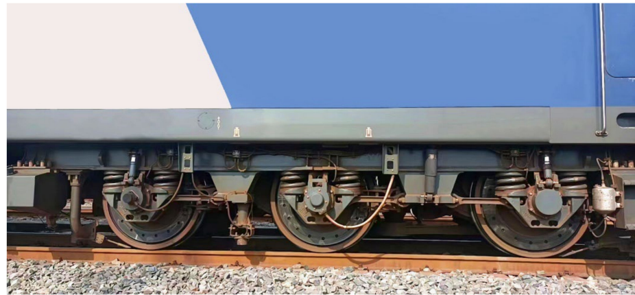
Figure 6. The locomotive bogie in refurbishment test after the operation.
