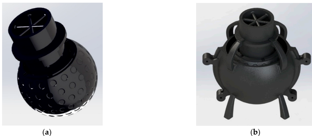
Figure 9. Fabrication of the rotor bowl: (a) the ABS inner structure of the rotor around which epoxy is cast; (b) the two-part mold assembly surrounding the inner structure.
