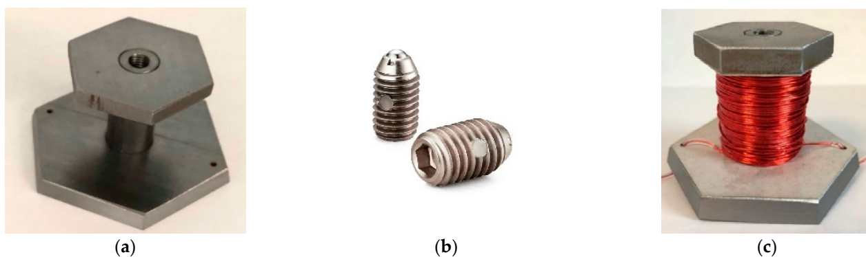
Figure 4. Stator poles and bearings: (a) assembled regular hexagonal pole unit showing tapped M6 threading for Hudson bearings; (b) M6 Hudson bearings assembled into the hexagonal poles; (c) wound stator pole ( N = 522 turns of 24 AWG magnet wire).
